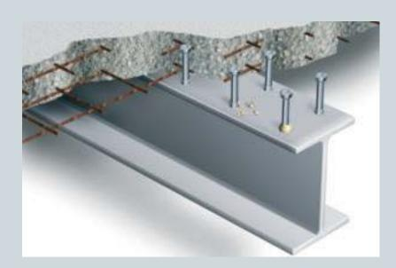
Shear connector application in steel composite construction.
