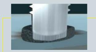
As a result, an even joint is achieved with a strength which is above the strength of stud and base material.
