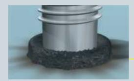
The molten areas solidify. The short and clean welding process does not require any machining.
