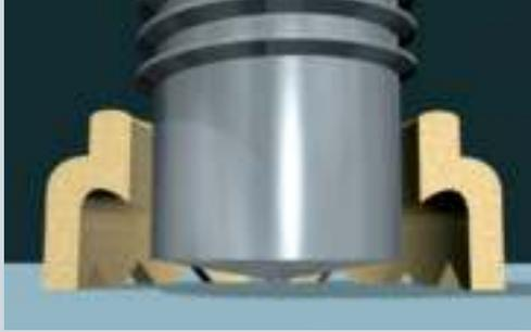
**Welding process with ceramic ferrule: Joining of stud-type welding elements with a diameter 2 to 25 mm (M24) onto thicker sheets of about 2 mm or higher. Mild steel and stainless steel.**
