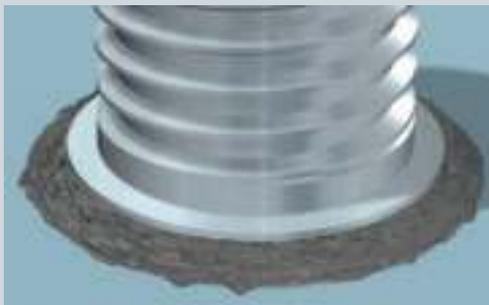
The molten areas solidify. The short and clean welding process does not require any machining.
