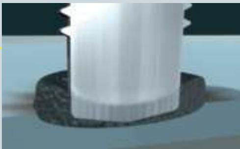
**As a result, an even joint is achieved with a strength which is above the strength of stud and base material.**
