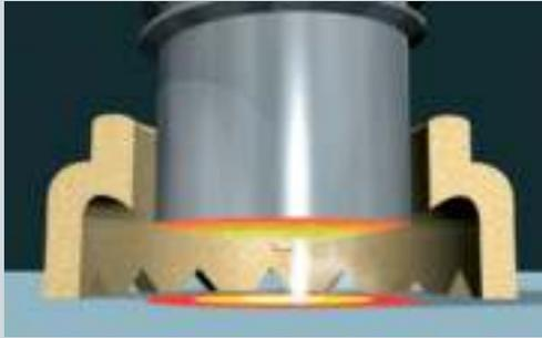
**The welding stud is lifted and a secondary arc (pilot arc) of low current is ignited between stud tip and work piece.**
