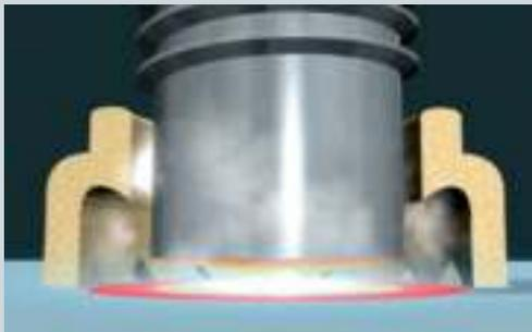
**Then the ignition of the main arc is carried out. Stud and work piece are melted. The stud is moved to the work piece, the two molten zones join.**
