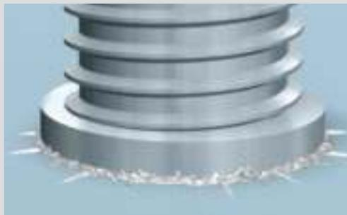
**The molten areas solidify. The extremely short and clean welding process does not require any machining.**
