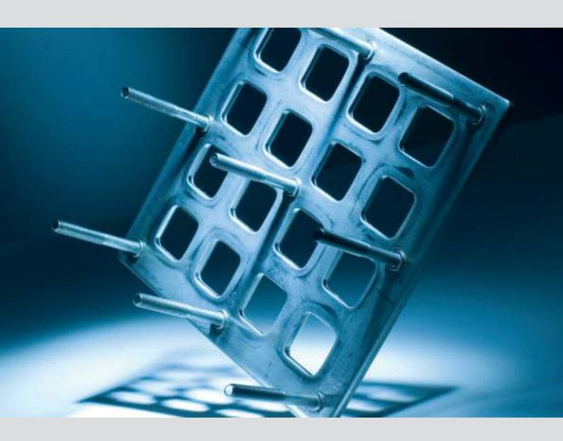
Capacitor discharge stud welding
