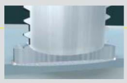
As a result, an even and complete joint is achieved with a strength which is above the strength of stud and base material. The low thermal load provides welding onto thin sheets without damage to the rear side.
