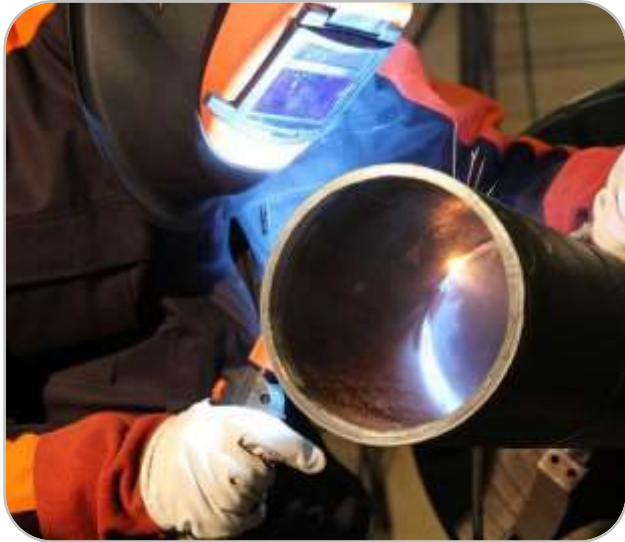
Fig. 2. WiseRoot+ welding process.
