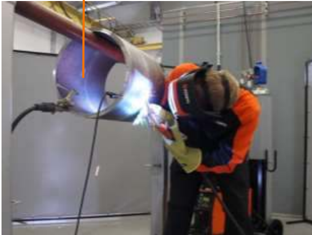
Fig. 8. Fixed pipe welding.
